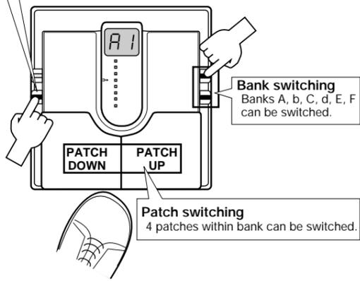
Bank/patch switching when Bank Hold is on
