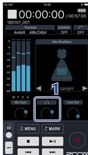
1. Drag the headphone volume on the Home Screen up and down to adjust the level.
