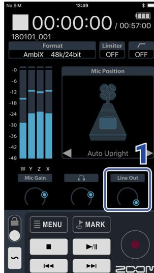
1. Drag the Line Out level on the Home Screen up and down to adjust the level.
