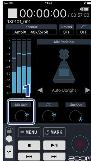
1. Drag the Mic Gain on the Home Screen up and down to adjust the level.
