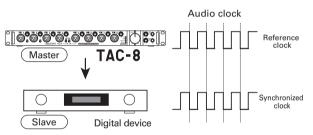
The **TAC-8** is operating as the master, and the audio clock of the **TAC-8** and the other digital device are synchronized.
